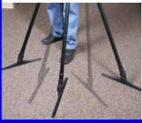
The patented Sidewinder tool series was developed by an ex-perienced contract cleaner seeking to increase his associates productivity by changing from the traditional push pull motion utilized with conventional cleaning nozzles to a vertical design which accommodates sweeping in an arc similar to what one would have done when mopping.
